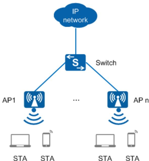
Starting from V200R020C10, some AP models running in Fat mode (depending on actual specifications) also support the leader AP networking and can manage a small number of Fit APs, thereby implementing small-scale batch deployment and simple O&M of basic WLAN services.
